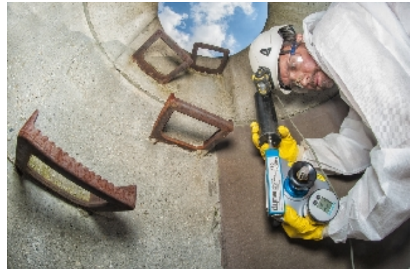
Tensile adhesion test on a coated manhole
