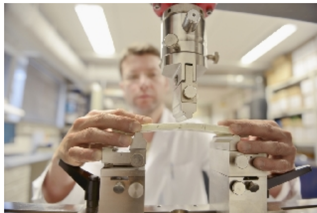
Three-point bending test on a CIPP-Liner
