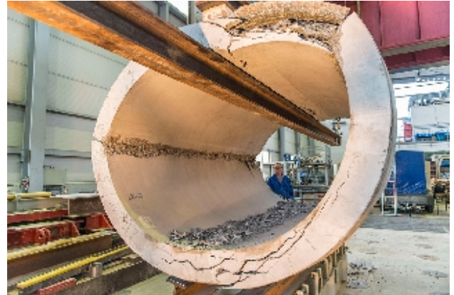
Vertical compression test on a reinforced-concrete pipe
